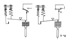
Set point and reset point must be between 10% and 90% of the selected scale.
